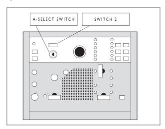
Figure 1.3 Under-panel controls on the LBB 3222/04 interpreter desk
